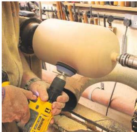
▲ Pic.23 Keep the drill down low. Sanding on the lower quadrant with a small gap at the top of the pad means that the drill will be easier to control
